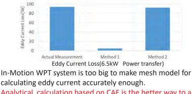
Analytical calculation based on CAE is the better way to analyze eddy current loss of in-motion WPT system.
